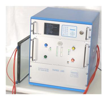
This gas filling machine has been developed for an economical gas filling process. The capacity is approximately Up to 900 units per day – with one filling-line
