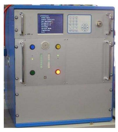
This gas filling equipment has been developed for an economical gas filling process. The capacity is approximately 500 units per 8 hours/day for one line  $(0.8 \text{ m}^2 - 14\text{mm} - 11.2 \text{ litres volume})$ . Upgrading is possible to 4 lines, which means you get a capacity up to 1500-2000 units per day.
