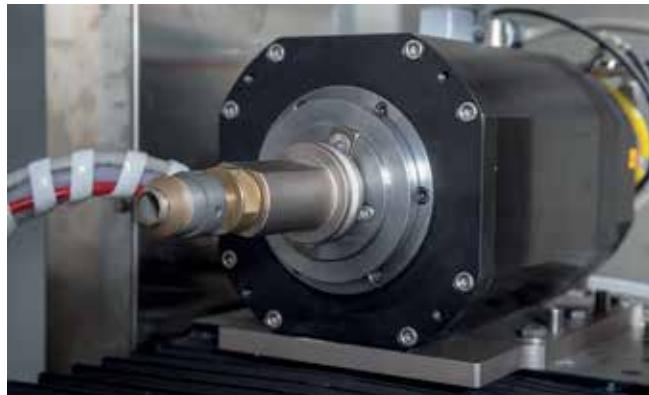
Highly precise electric spindle with an ISO 30 cone with pressurization system. Rotational speed up to 10,000 rpm.
