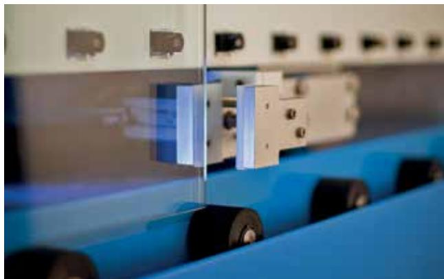
High precision thanks to the measuring system of the real position of the glass through magnetic bars, guaranteeing an accuracy of  $\pm 0,15\text{mm}$  over time.
