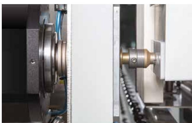
Automatic measuring system of the tools, which can be operated manually or automatically after a predetermined number of drilled holes, compensates for tool wear automatically.
