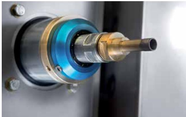
Spindle with rotational speed up to 6000 rpm. Management of the working pressure of the tool with a hydropneumatic advancement system for the Z-axis. This adapts the penetration speed in conjunction with the effective sharpness of the tool.
