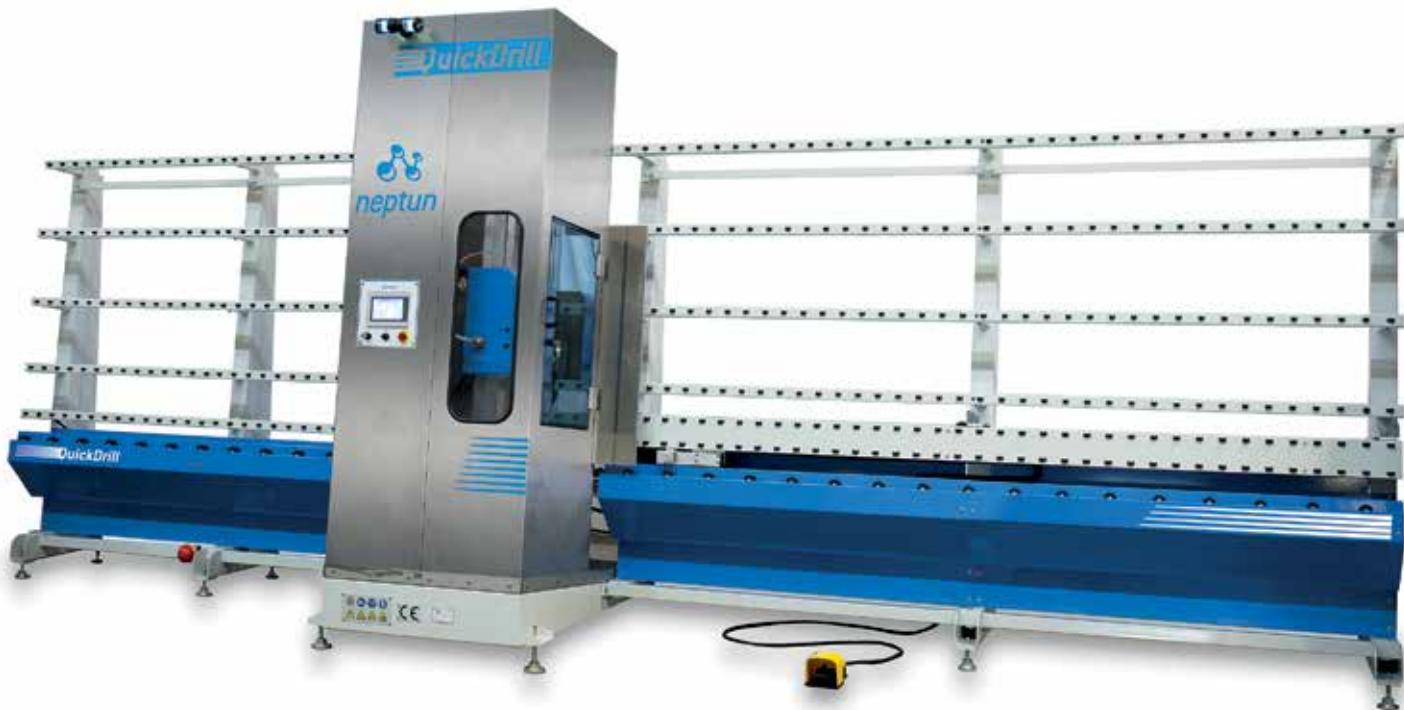
A vertical CNC machine for **drilling** and **countersinking** holes.
