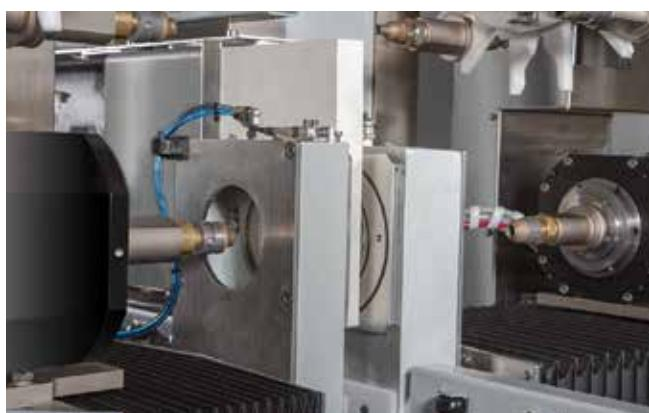
The automatic dressing system allows the restoration of the sharpness of the tools in a short time in a completely automatic way.
