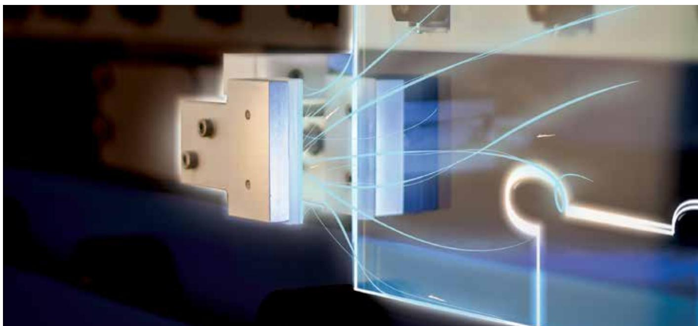
**Quickline** consists of **two** modules: **QuickDrill** for holes and countersinks and **QuickMill** to process notches, hinge cut outs and internal portholes. Both modules can operate over the entire working area with high no restricted zones, with high speed and precision. The main benefits of the Quick machines are their **high processing speed and precision**.
