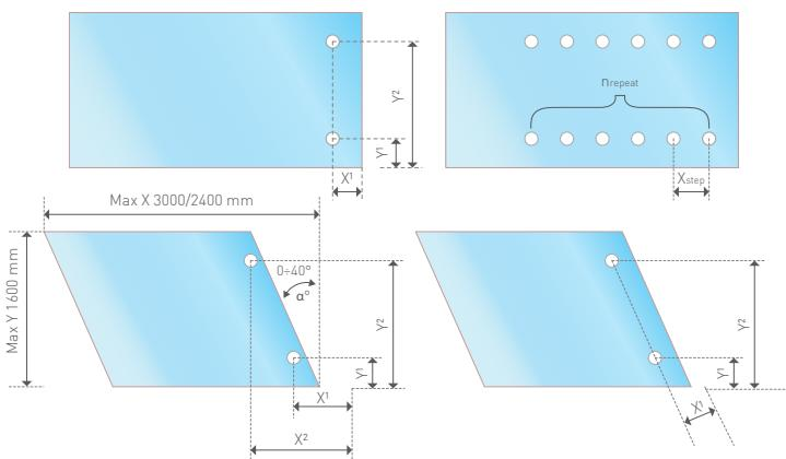
Powerful function of nested programs, allowing their recall and repeat "n" times after definition of the parameters.
