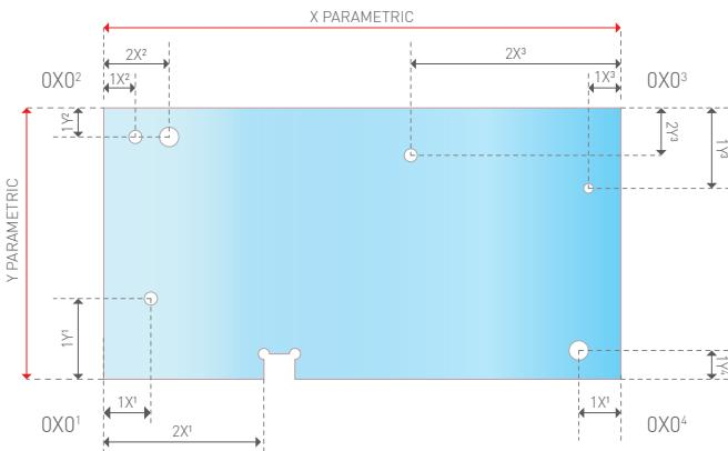
The reference points for the positioning of the shapes can be chosen without any limitations. This allows to create models for **complete parametric doors**, which can quickly be applied to glass sheets with different dimensions; every processing can be given a different reference point. It is also possible to manage out-of-square pieces up to 40°.
