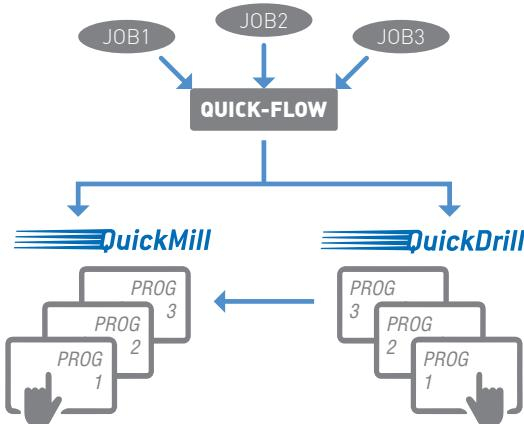
**QuickFlow** is a superior programming layer which brings the machines together, directing the entire process and creating sub-programs into the separate machines, one for milling and one for drilling. In this way, both drilling and milling can be undertaken at the same time, yet autonomously, even with two separate glass sheets.
