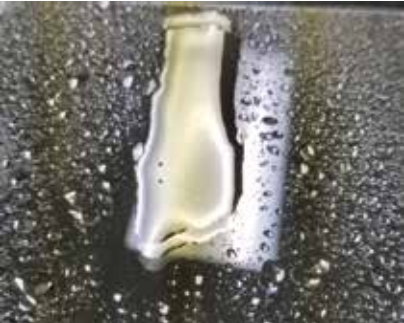
Diamon-Fusion®- Clear Fusion PRO Visible wear after 3,500 abrasion cycles Fail
