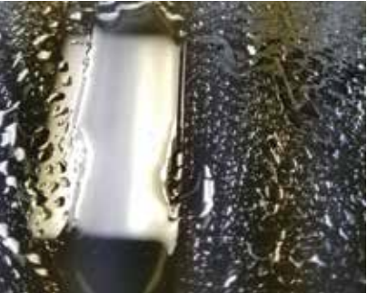
EnduroShield® Glass Coating Visible wear after 1,000 abrasion cycles Fail
