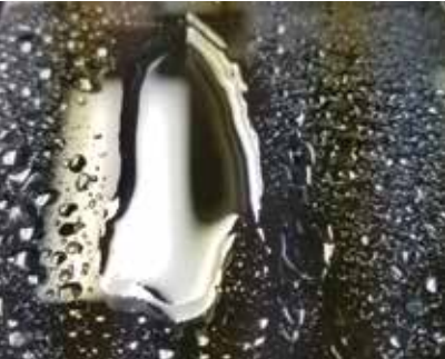
Ritec ClearShield® Glass Protect Visible wear after 2,500 abrasion cycles Fail
