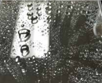
Invisible Shield® PRO 15 Glass Coating Minimal wear after 5,000 abrasion cycles Pass
