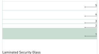
The production of laminated security glass requires one (1) side coated LUXAR®. The uncoated surface will be towards the inter-layer or resin, while the anti-reflective coated surface will be
